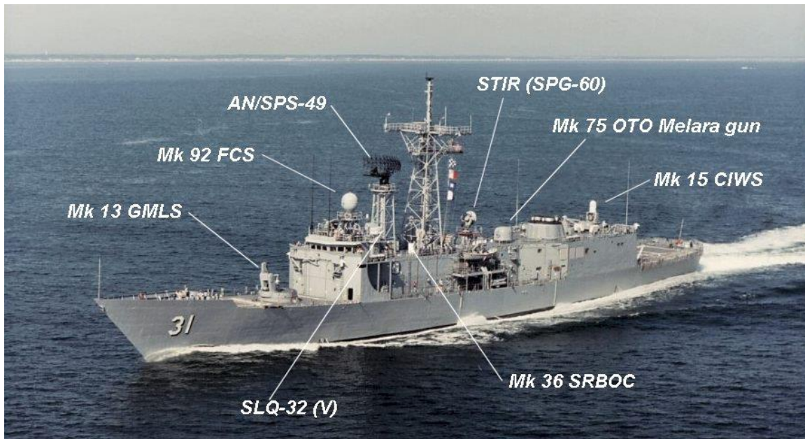
Above: USS STARK (FFG-31) with the various anti-ship missile defense systems identified. (Photo: U.S. Navy, notations Bob Stoner)
