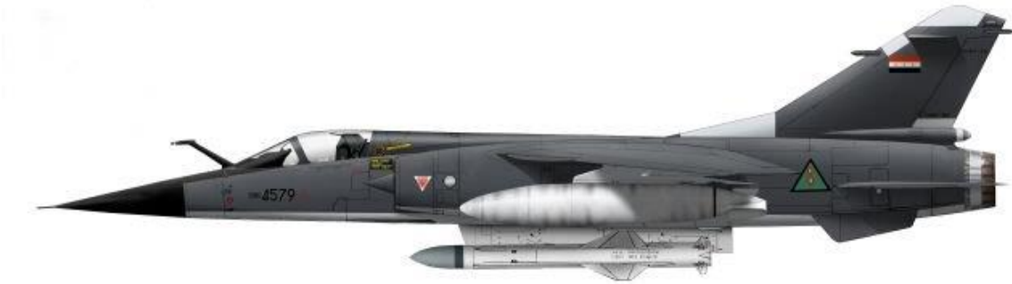
Above: An Iraqi Dassault F.1EQ-6 configured for maritime strike with the MBDA AM39 Exocet air-launched anti-ship missile. (Art: ACIG.com)
