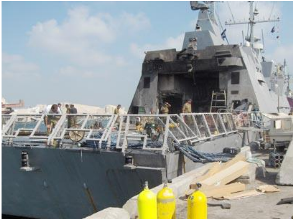
Above: HANIT alongside the pier at the Israeli Ashdod Naval Base. Fire and blast damage is apparent to the helicopter hangar and starboard side hatch. (Photo: Israeli Navy)
