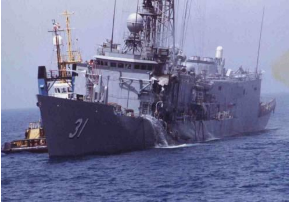
Above: STARK, with an ocean-going tug alongside for assistance. The fires just about extinguished and dewatering of flooded spaces is underway. (Photo: Navysite.de)
